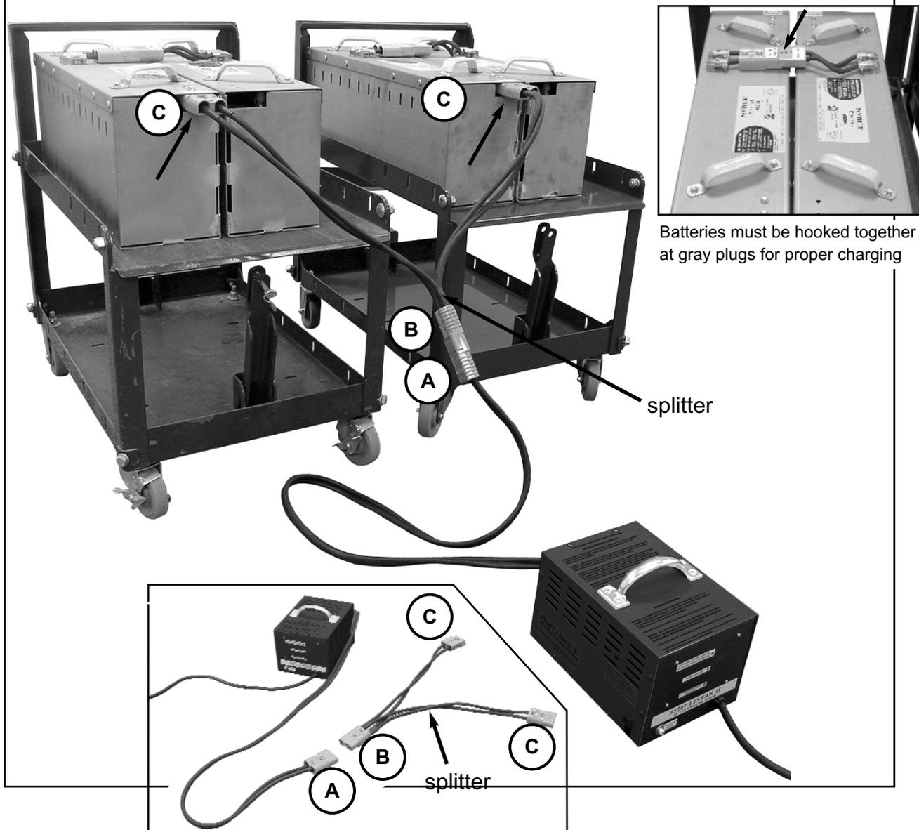
When charging in this manner, it works best when both 48 volt power packs are at the same level of discharge. Connect splitter plug (B) to charger plug (A). Connect splitter (plugs) (C) to each power pack. Make sure all connections are fastened securely. Once charger and splitter are connected to both power packs, connect charger to power source. Complete the charging sequence.
