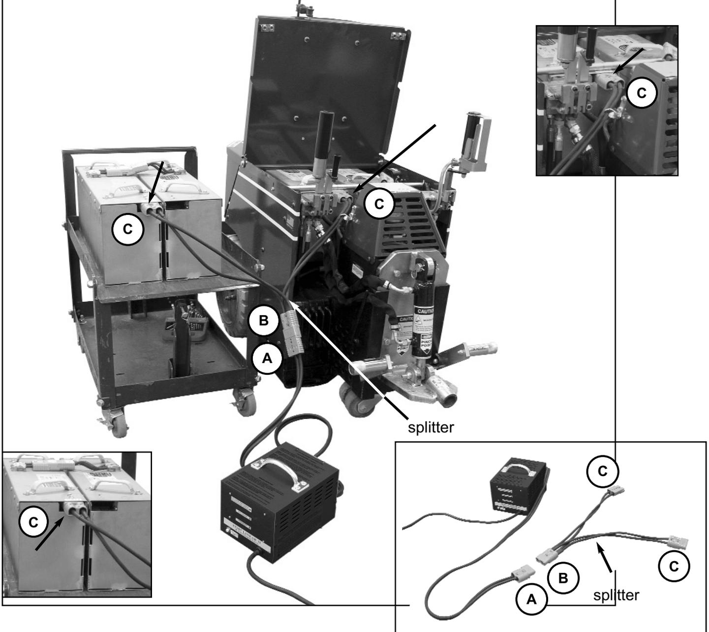
When charging in this manner, it works best when both 48 volt power packs are at the same level of discharge. Connect splitter plug (B) to charger plug (A). Connect splitter (plugs) (C) to each power pack - one in machine and one on cart. Connect charger to power source. Complete the charging sequence. Charging will take 4 to 8 hours depending on the level of discharge of each power pack. The lower the voltage, the longer it will take to restore the power pack.
