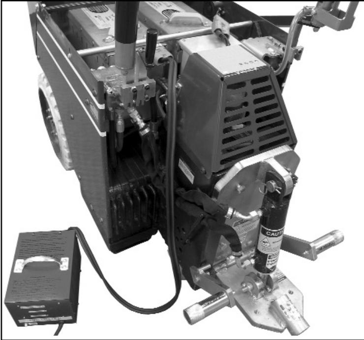
Charging time: range 2 to 4½ hours depending on the level of discharge of the power pack.
